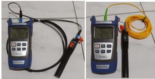
(a) Kabel FO drop core (b) Kabel FO patch core Gambar 4. Pengukuran kabel FO Drop Core dan Patch Core
